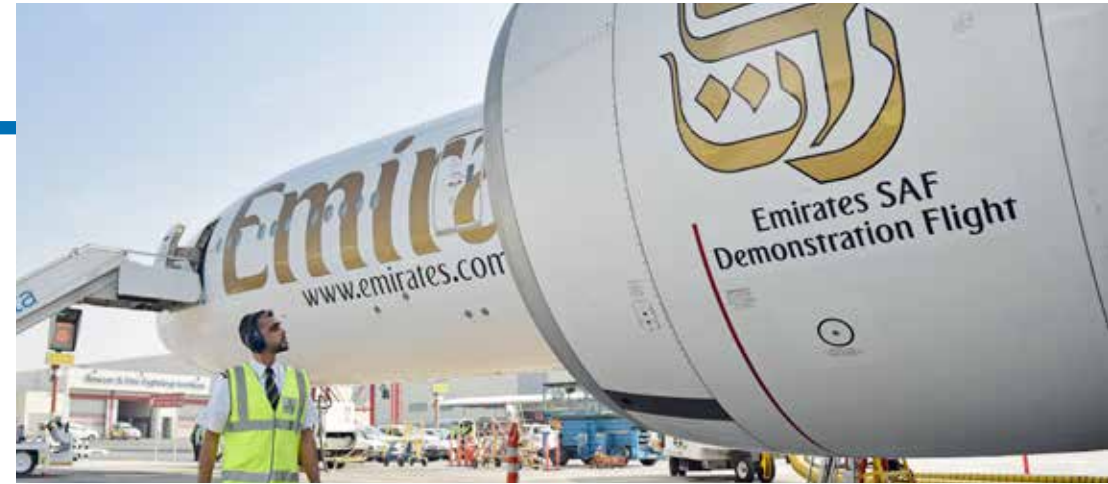
The Emirates flight test utilized 18 tons of SAF in one engine of a 777-300ER blended from two producers, Neste and Virent. The flight flew over the Dubai coastline for just over an hour. (Emirates photo)
