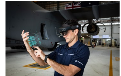
Boeing Defence Australia C-17A maintenance operations planning analyst Jared Parker tests Boeing's augmented training operations and maintenance solution. It allows aircraft technicians to perform critical maintenance on the Royal Australian Air Force's giant cargo workhorse, the Boeing C-17 Globemaster III, remotely from anywhere in the world — viewing real-time, hands-free, interactive 3D holograms right before their eyes.
