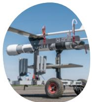
**2020** In situ completed the first flight of their ScanEagle3 unmanned aerial vehicle powered by an all-electric, hydrogen fueled, proton exchange membrane (PEM) fuel cell.
