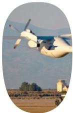
**2012** Boeing's Phantom Eye high-altitude and long-endurance uncrewed aircraft flew several flights in California powered by liquid hydrogen.
