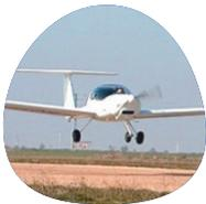
**2008** Boeing's Fuel Cell Demonstrator, a two-seat Dimona, flew three flights in Spain—representing the first piloted airplane in history to use power generated solely by hydrogen fuel cells.
