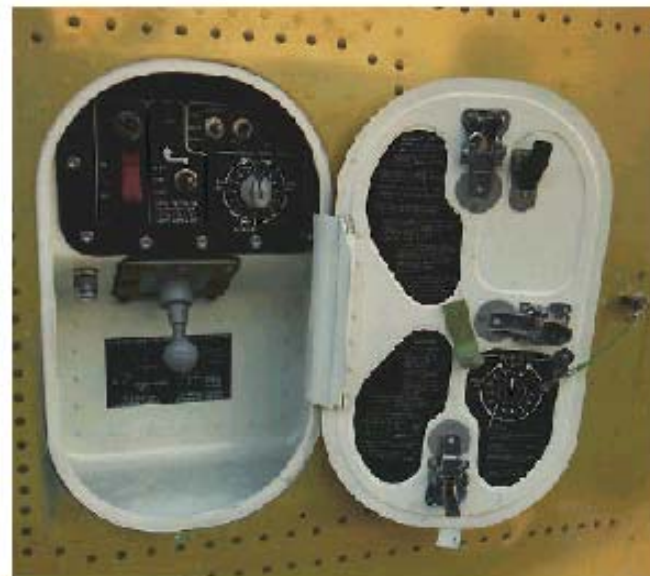
Cargo door/handling system control panel
