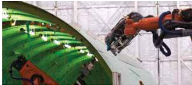
FIGURE 39. The Boeing 777 FAUB fuselage assembly process.
