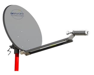
The 98cm Ka-Band Terminal is a professional grade product suitable for Enterprise applications. It is made up of a 98cm steel antenna and integrated transceiver and has a standard IF interface common to industry standard VSAT modems. Full Ka-Band transmit coverage from 29 to 31 GHz with flexible polarization for truly global operation (5W option only). The SKY 98 is pre-approved for out-of-the-box compatibility with Inmarsat's Global Xpress Ka-Band network.
