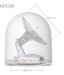
Downlink freq 19.2 to 20.2 GHz Uplink freq 29 to 30 GHz ICM: module iDirect (NTG-249) Block up convertor 5W Elevation range -20 to 115° Azimuth range 360° Temperature: -25° to 55°C
