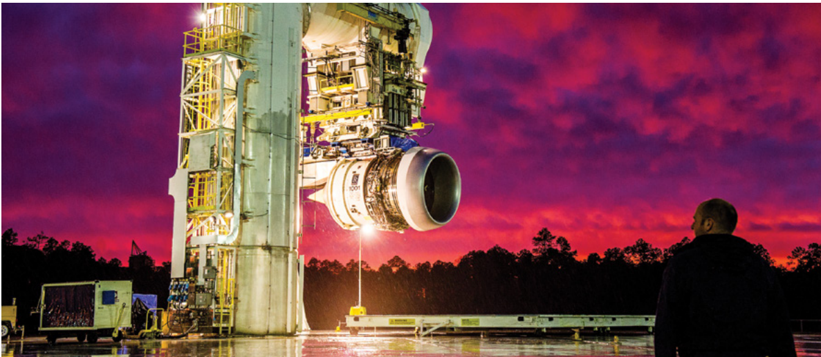
Boeing tests advanced jet engine technology at NASA's Stennis Space Center in Mississippi. Innovative applications of materials such as composite matrix ceramics will make engines quieter, lighter and more efficient. (Boeing photo)
