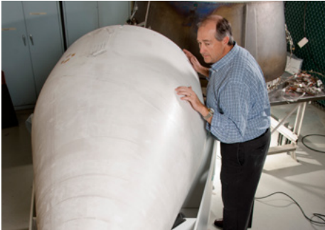
Engineer Craig Wilsey inspects an engine nozzle made of composite matrix ceramics. (Boeing photo)
