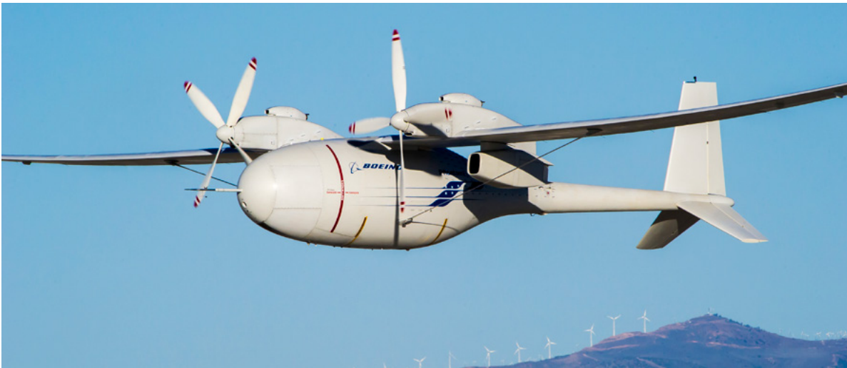
The Phantom Eye is a long-endurance unmanned vehicle designed to stay airborne for up to four days powered by clean-burning hydrogen, which leaves only water in the atmosphere. (Boeing photo)
