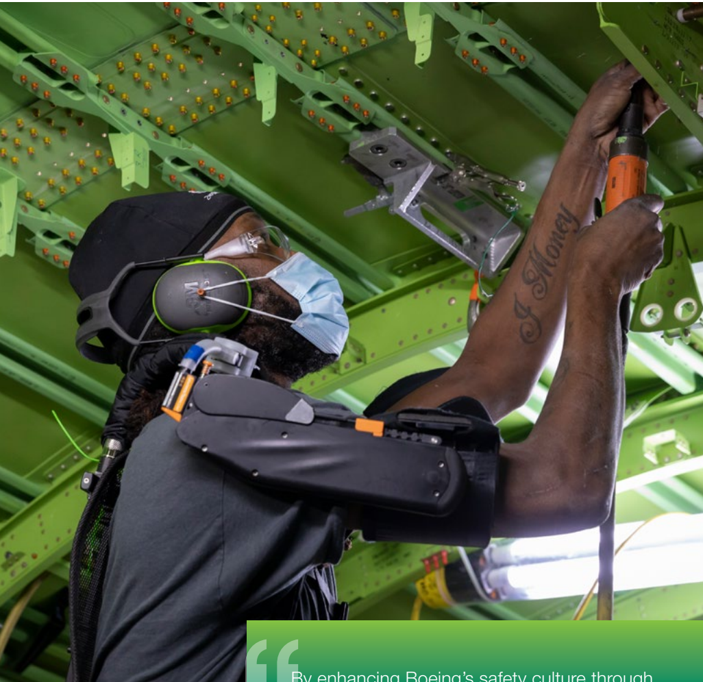
Working on a 767 in Everett, Washington, mechanic Jason Turner is much more comfortable thanks to a shoulder support exoskeleton. (Boeing photo)
