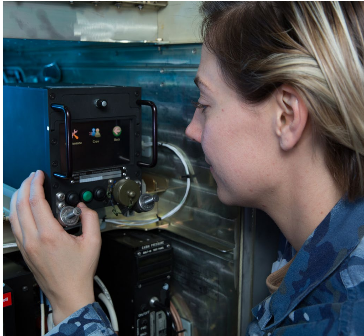
An aviator with the Royal Australian Air Force performs system checks on a C-17 with Boeing's Aircraft Data Reasoner. (RAAF photo)
